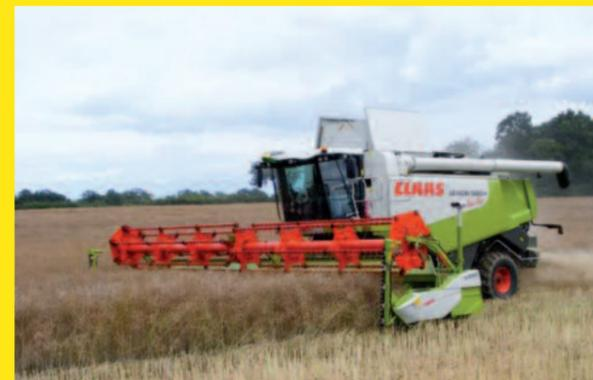
Claas Lexion 580 uses 50l/ diesel hour
