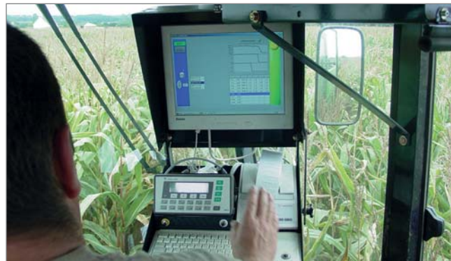
Online NIRS systems on trials harvesters enable quality assessments to be made as plots are harvested.
