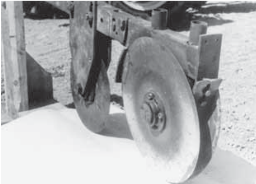
Fig. 4.4. A typical triple disc no-tillage opener that forms a V-shaped slot (from Baker, 1976b).
