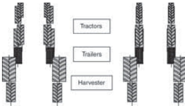
Fig. 16.4. Placing all the equipment in the example around a common centre line (left) shows that it is only the harvester that has a significantly different track width. Available settings on the tractors will allow them to be aligned with the trailers, as indicated on the right, with only the cost of time.
