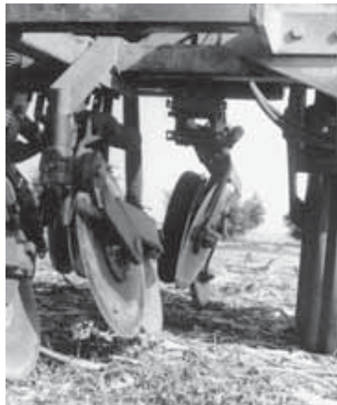
Fig. 4.8. A pair of slanted discs at opposing angles. The front discs place fertilizer and the rear discs place seed at a shallower depth. (From Baker et al. , 1996.)
