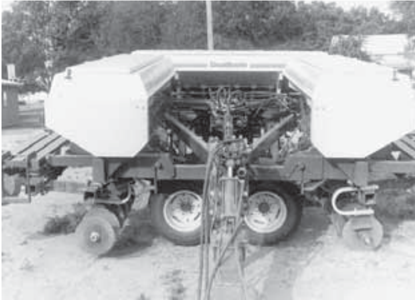
Fig. 13.10. A folding arrangement for multiple drills.
