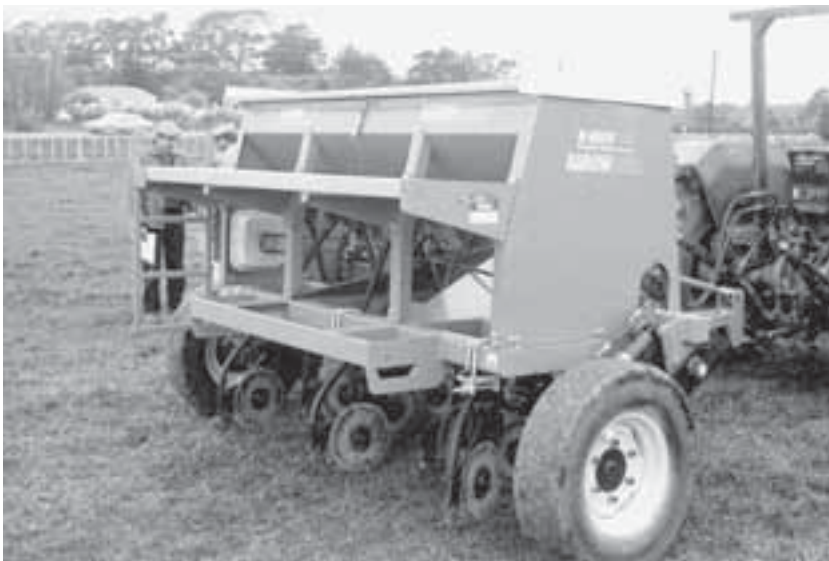
Fig. 13.12. A no-tillage drill with elevated product hoppers.
