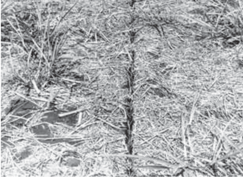
Fig. 7.1. Class IV slot cover remaining intact after passage of a winged opener, equipped with scrapers (inverted-T-shaped slot), through a damp sticky soil (compare with Fig. 4.5).
