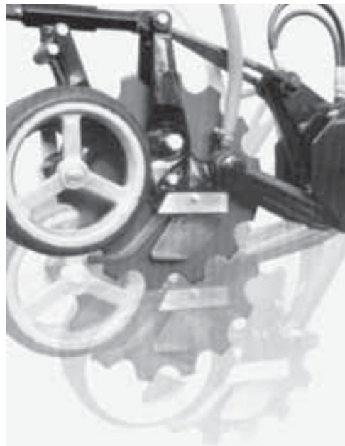
Fig. 8.10. A winged no-tillage opener mounted on parallelogram drag arms and pushed down with a gas-over-oil system, showing its extraordinarily large range of vertical travel, which is important in no-tillage.
