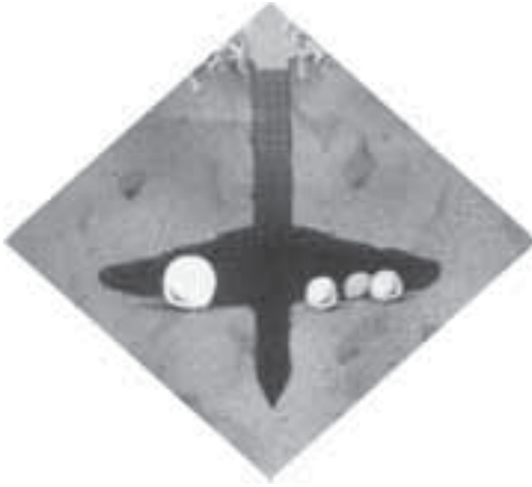
Fig. 4.28. Horizontal separation of seed and fertilizer by the disc version of a winged opener.
