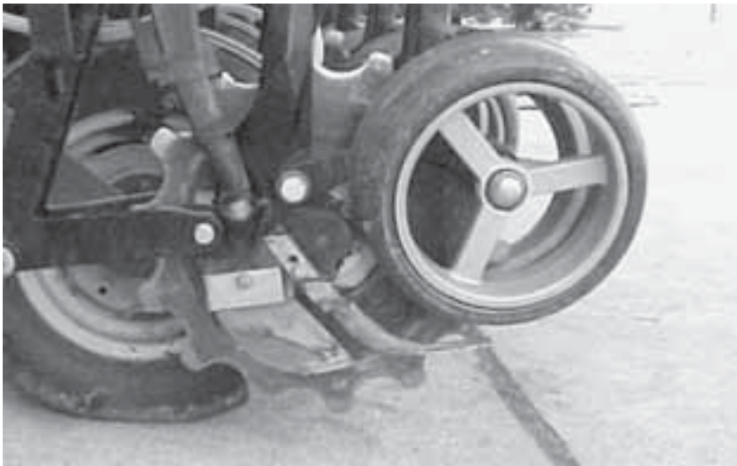
Fig. 10.20. Underground scrapers on the disc version of a winged no-tillage opener.
