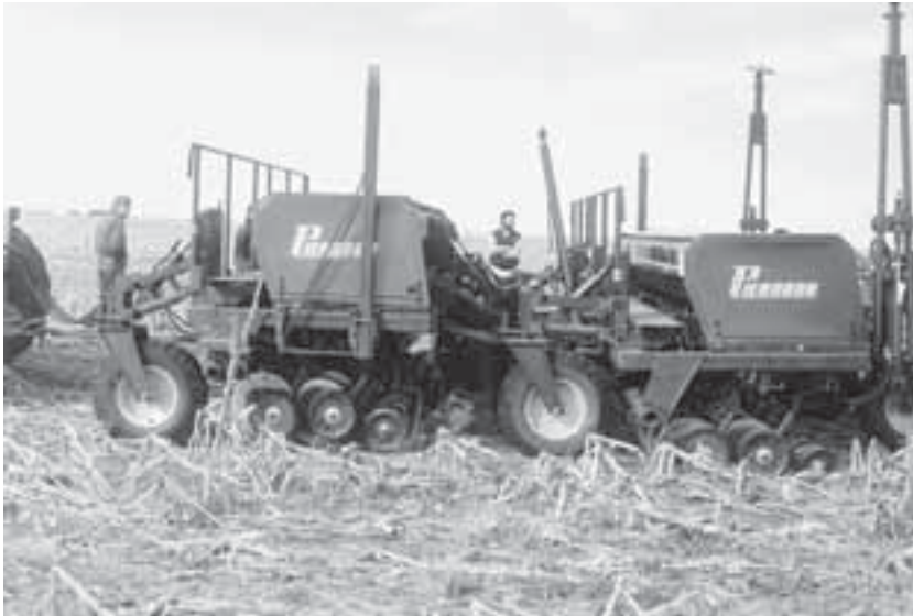
Fig. 13.9. Two-wide row units arranged in tandem to produce a drill with half-row spacing.
