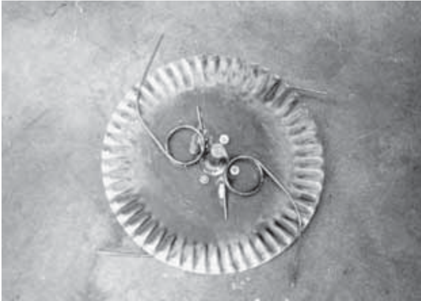
Fig. 10.17. A flicking device designed to self-clean stationary tines.
