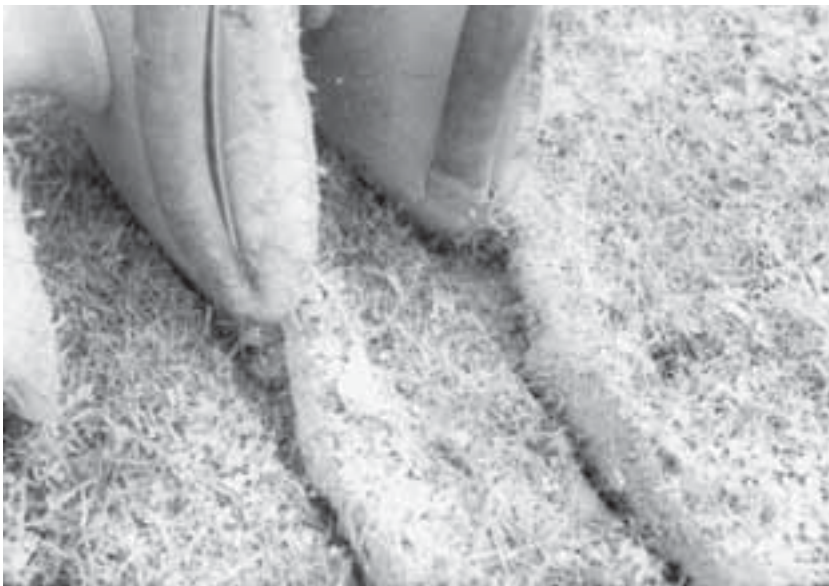
Fig. 4.10. An angled dished disc no-tillage opener (from Baker et al. , 1996).
