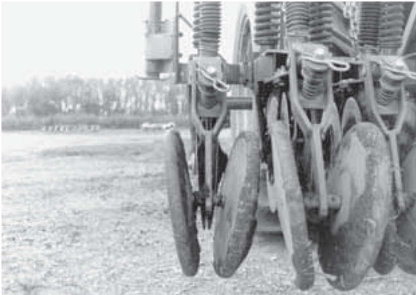
Fig. 4.7. Press wheels arranged in a V configuration for closing no-tillage slots created by vertical double disc openers (from Baker, 1981a, b).
