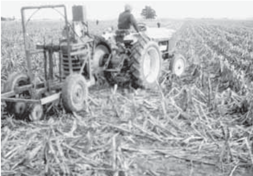
Fig. 19.14. A single-row machine for testing the residue-handling capability of a no-tillage opener.
