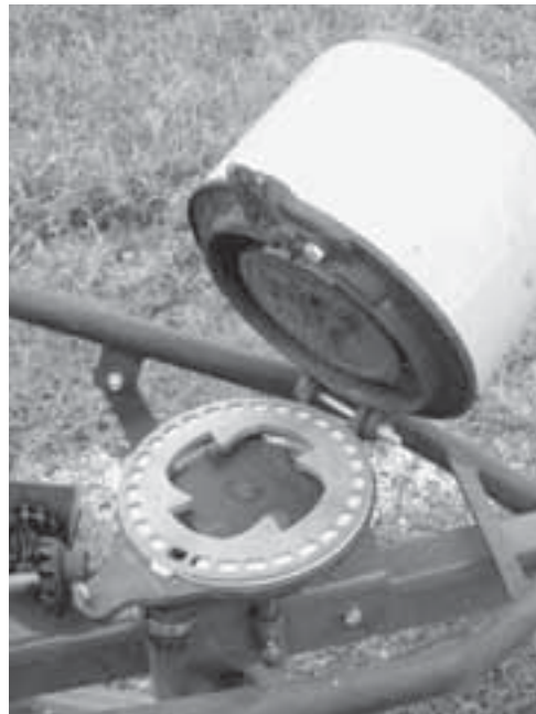
Fig. 14.7. A closed hopper system for easy seed plate change.
