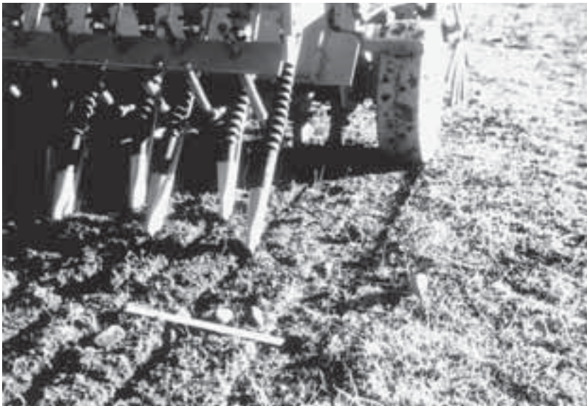
Fig. 4.16. Narrow tilled strips left by a power till 'no-tillage' opener (from Baker et al. , 1996).
