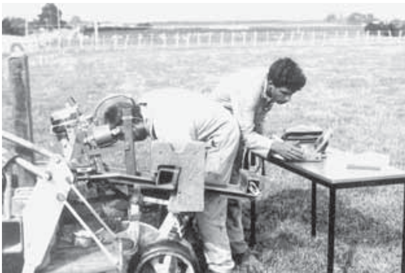
Fig. 19.10. A test stand for monitoring disc drag of a no-tillage opener.
