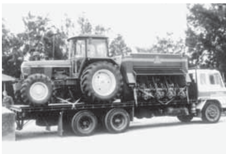
Fig. 19.17. A fully self-contained drilling machine for field testing and on-farm demonstrations.
