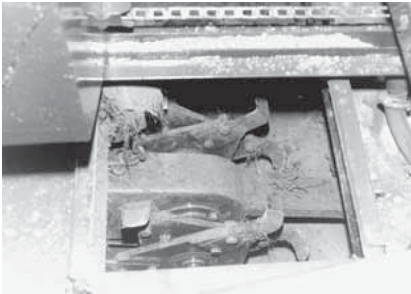
Fig. 4.18. Power till no-tillage openers arranged in pairs (from Baker, 1981a, b).
