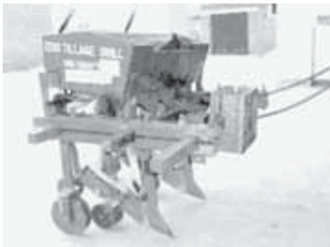
Fig. 14.19. A zero-tillage flat-type toolbar showing the mounting plate for a two-wheeled tractor.
