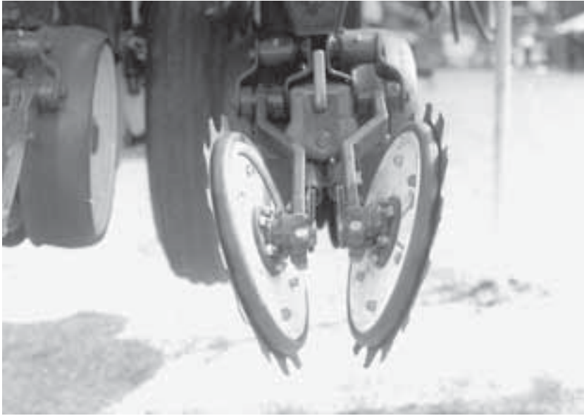
Fig. 5.11. A pair of combined spiked discs and angled press wheels for covering no-tillage slots (from Baker et al. , 1996).
