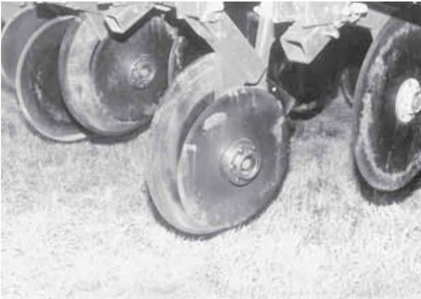
Fig. 4.3. Typical unequal-sized double disc no-tillage openers that create vertical V-shaped slots.
