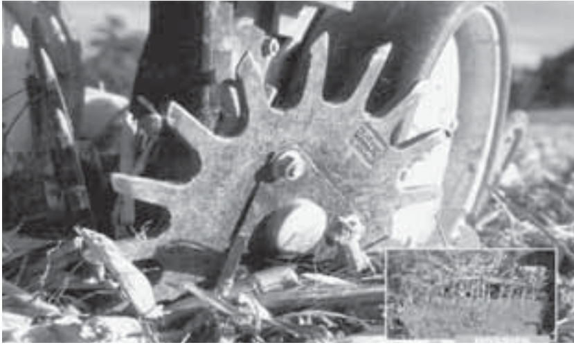
Fig. 10.10. A pair of synchronized star wheels (row cleaners) for pushing residues aside.
