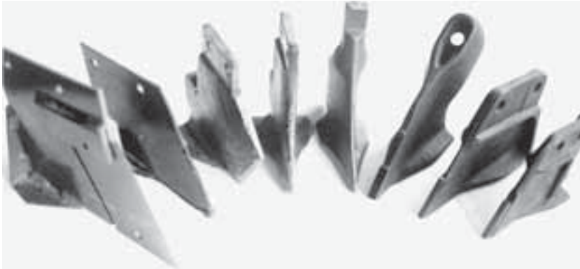
Fig. 4.23. Several versions of the 'Baker boot' inverted-T-shaped no-tillage opener (from Baker et al. , 1996).
