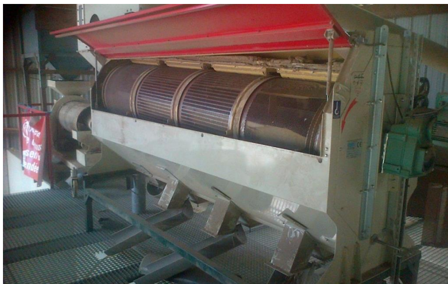
Figure 56: Rotary (Trommel) cleaner. Photo courtesy of www.arc2020.eu
