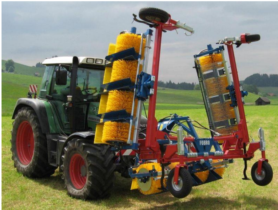
Figure 53: brush-weeder to control growth of undersown crops. Photo courtesy of www.Baertschi.com
