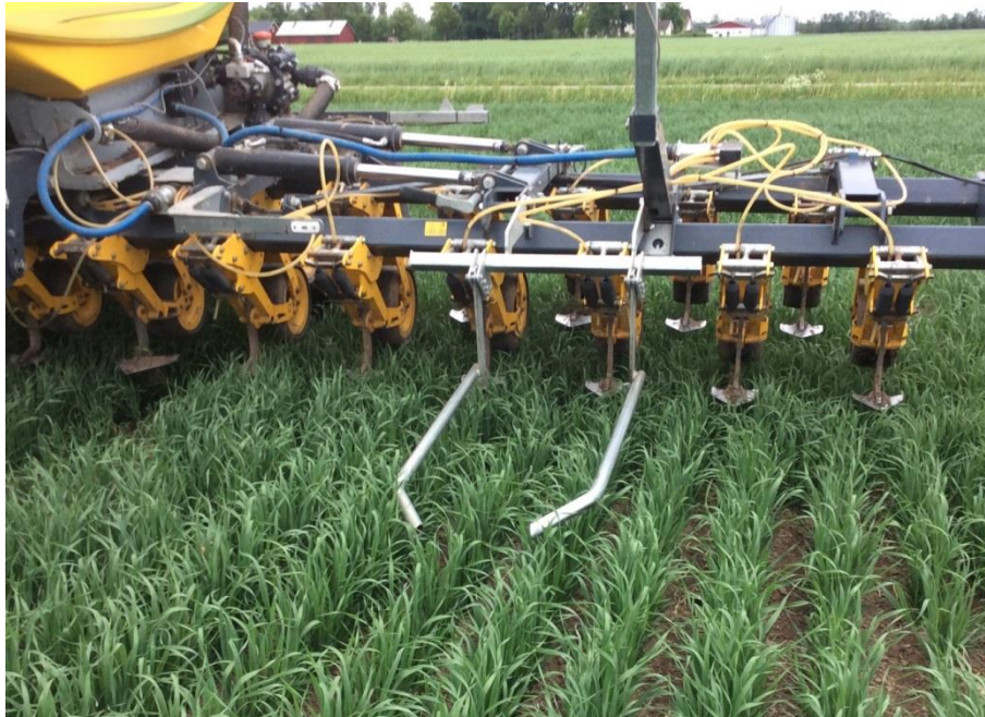
Figure 50: the System Cameleon about to hoe wheat
