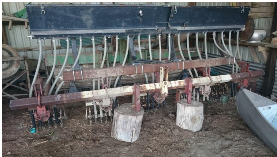
Figure 45: home made machine for interseeding maize
