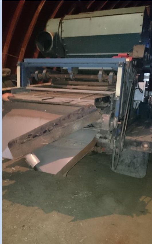
Figure 35: converted old Flaman 54" screen cleaner
