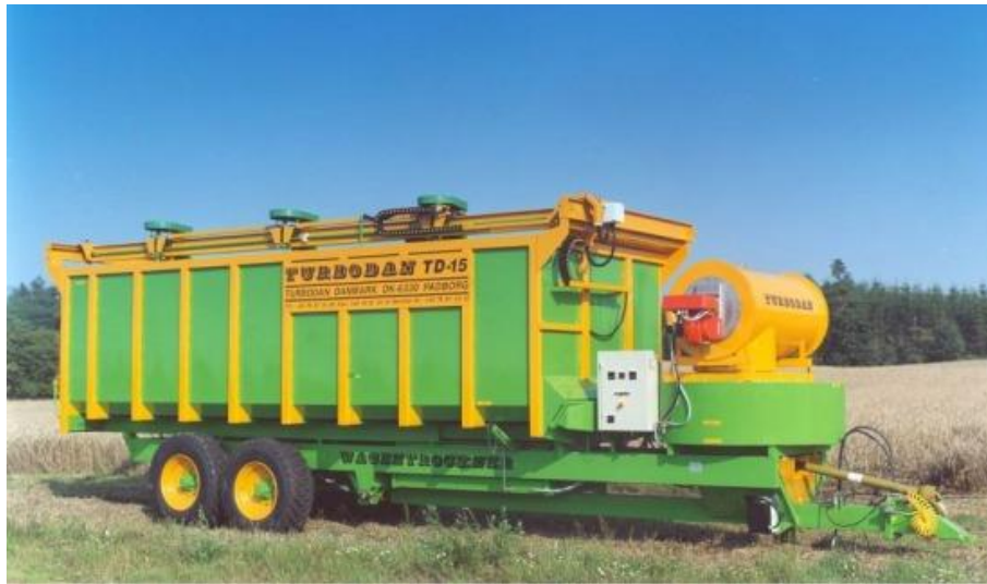
Figure 55: grain dryer trailer. Photo courtesy of www.agrozaibas.com
