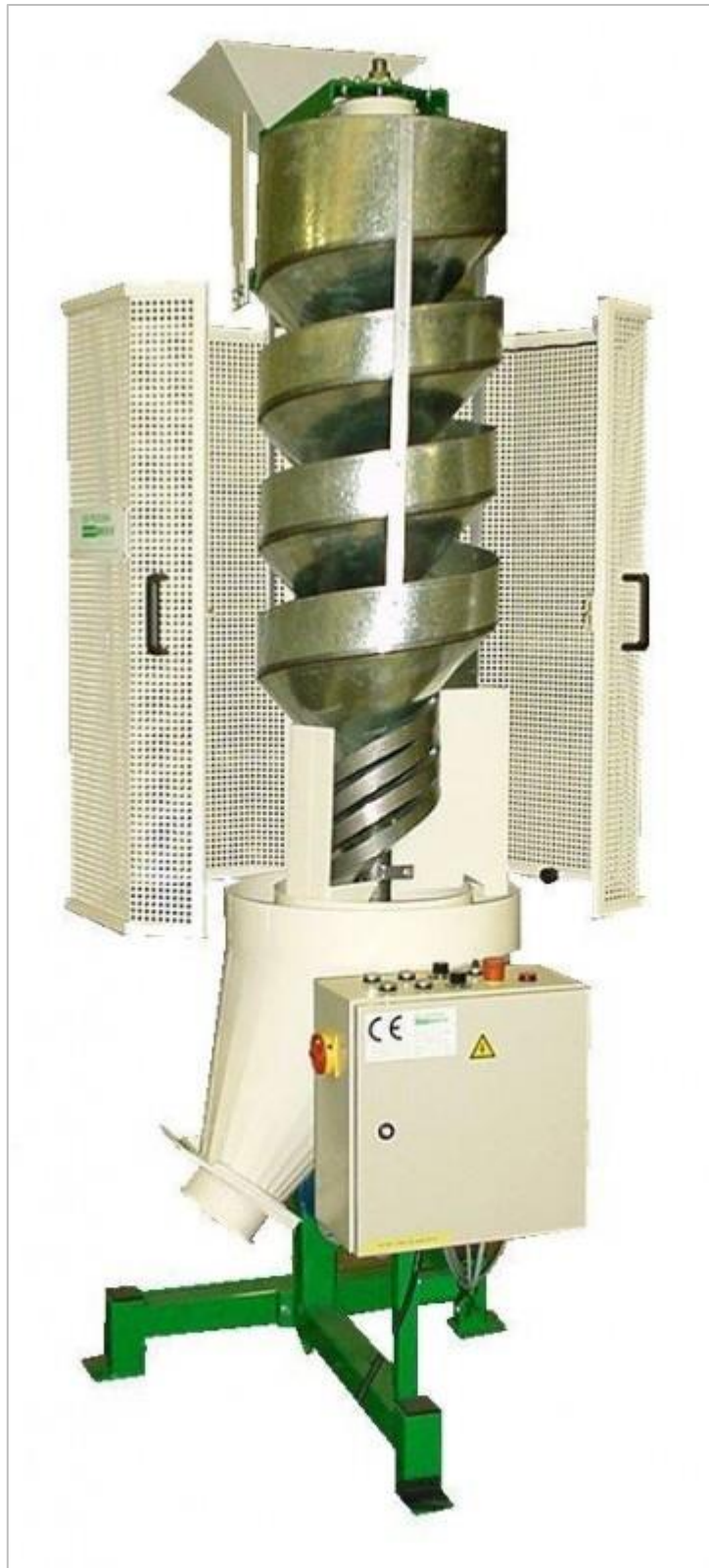
Figure 58: Spiral separator. Photo courtesy of www.seedprocessing.nl
