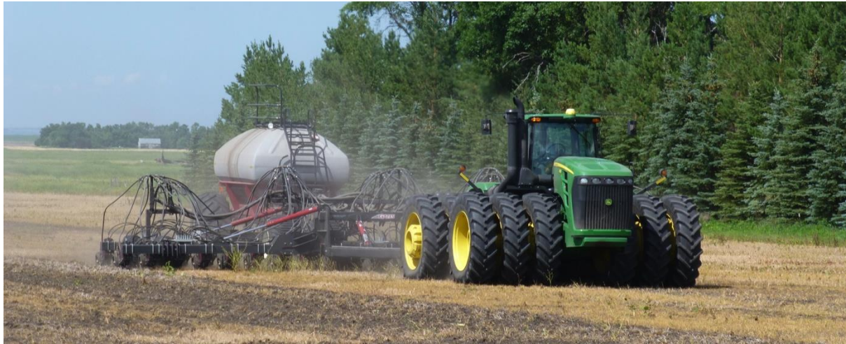
Kevin Larsons's 45ft Cross-Slot drill, which enables large acreages to be planted by one man
