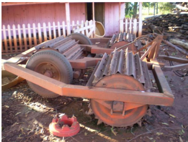
A home made crimper (knife) roller for destroying cover crops without herbicide.
