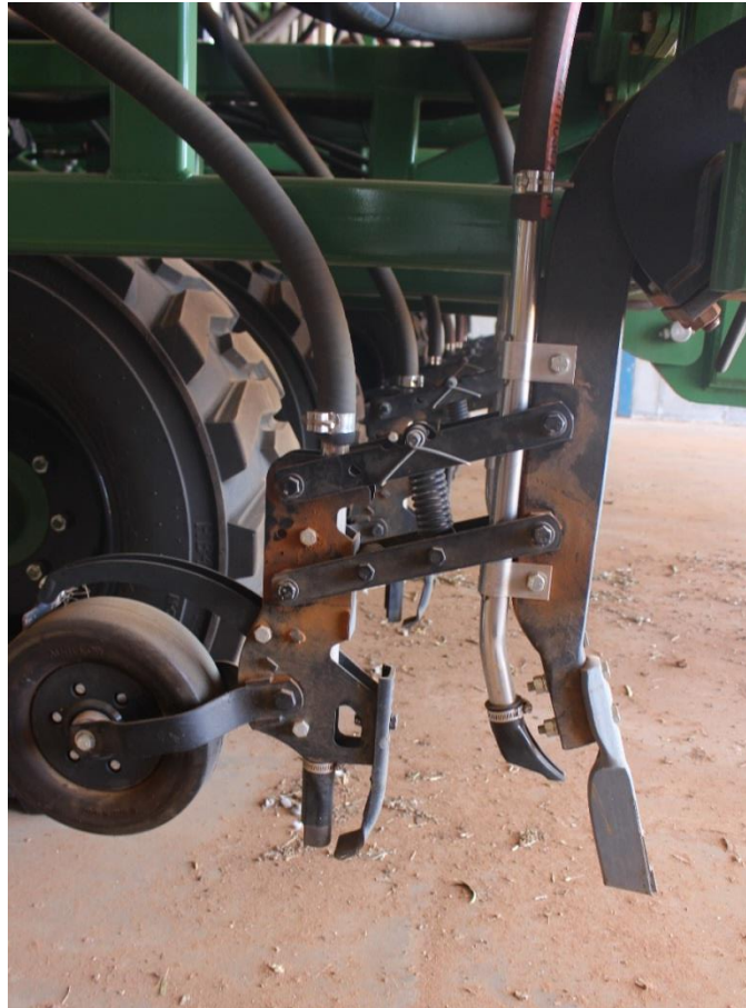
Figure 30. The popular DBS tool bar tine system favoured by Darren Longmire and others
