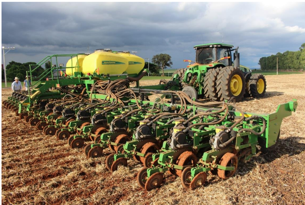
Figure 28. Corn planting on an angle after soya beans in Brazil; triple hoppers for seed and fertiliser
