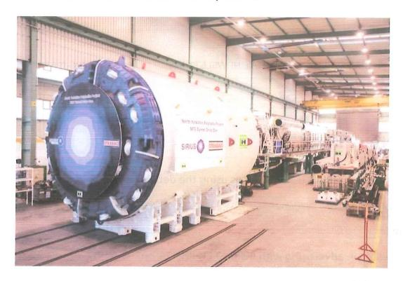
The first machine that will construct Sirius Minerals' underground mineral transportation tunnel between Whitby and Teesside has come off the production line.
