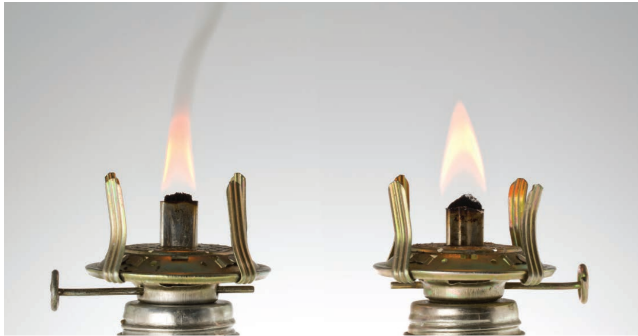
VISUALISATION OF SOOT BENEFITS. CONVENTIONAL DIESEL (LEFT) AND SHELL GTL FUEL (RIGHT)
