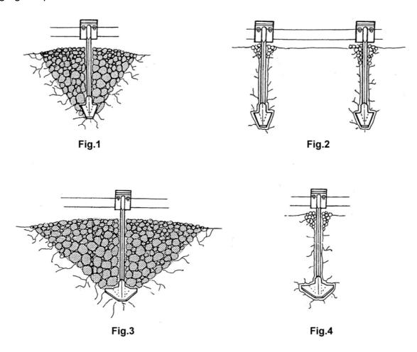
Figure 1 is the pattern produced by the narrow points and figure 3 is the pattern of the wide points – the wide points produce a much greater loosened area.
