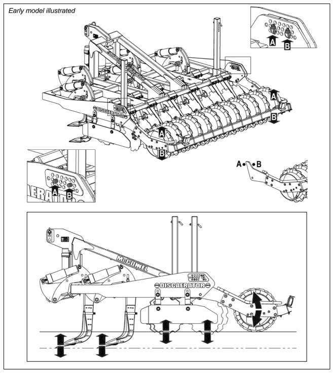
NOTE: It is advisable during transportation of the machine that the roller is 'locked tight' in position to avoid risk of the roller bouncing when travelling over rough terrain – this will reduce stress on components and increase stability of the carrying vehicle.
