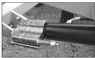
Ram Stops on early models are mounted adjacent to the ram and swivel over the ram rod to 'lock' the cylinder.
