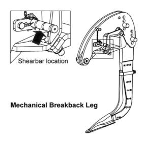
NOTE: It is important when replacing shear bars that genuine McConnel replacements (*Part No. 22520.54*) are used as these are specially designed to shear under a pre-determined force. Use of non-genuine parts will risk expensive damage to the machine and/or tractor. Under no circumstances should the shear bolt be replaced by a bolt or a metal rod.
