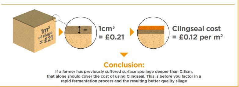
Clingseal is a flexible vacuum sheet that is used directly beneath traditional, heavier silage sheets. Clingseal clings more closely to the contours of the clamp surface and tuck in at the sides. This helps eliminate air pockets and provides a close fitting barrier to significantly reduce top and shoulder losses from aerobic spoilage.
