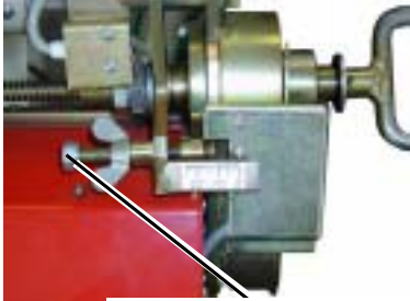
Adjusting setting screw for seed rate adjustment
