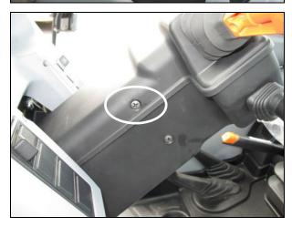
Remove the transmission forward/reverse lever.
