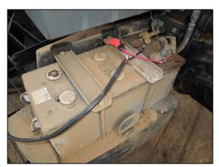
Example battery connection: MXM / TM series tractors
