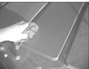
Allow the adhesive promoter to dry. Remove the backing tape from the foam strips and then apply the plate to the cab roof. Ensure that the foam strips make even contact with the surface. Apply pressure to adhere.
