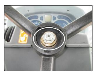
Soak the steering shaft splines with a spray penetrant or catalyst. Trimble recommends PB Blaster, available at www.pbblaster.com or your local automotive parts company.
