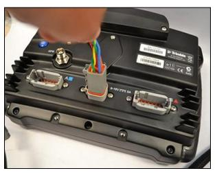
Step 4 Plug in the 12-pin CAN connection on P/N 75834.
