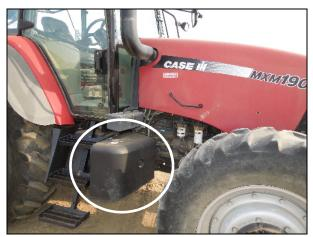
Example battery location: MXM / TM series tractors
