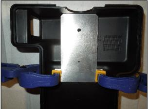
Drill a  $\frac{1}{8}$ " pilot hole into the plastic cover. Use the lower hole as a guide.
