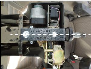
Bottom bolt aligned on centerline
