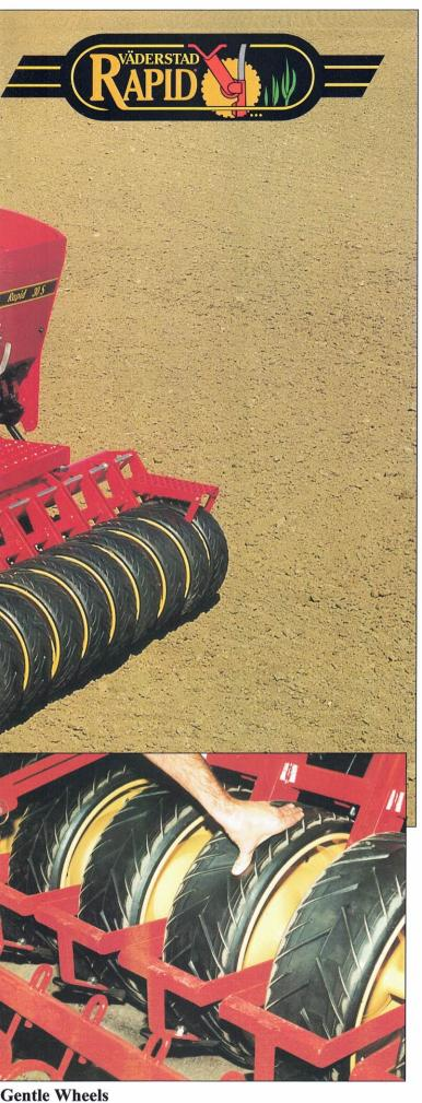
The drilling depth is governed by the back wheels from the top of the soil via a patented linkage system hooked up to two discs and coulters in front of them. The great flexibility in the tyres together with the scrapers prevents them from building up, even in wet conditions.
